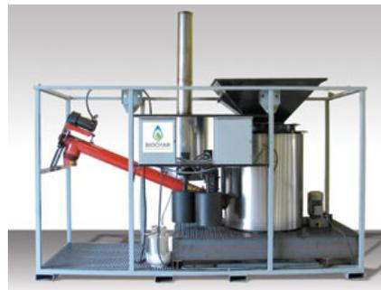
Biochar Engineering's Biochar 1000 can process 1,000 pounds of wood chips per hour. PHOTO: BIOCHAR ENGINEERING CORP.
